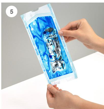
Allow the ink take effect on every seal seam for approx. 5 s. Check all seal seams for leaks.
