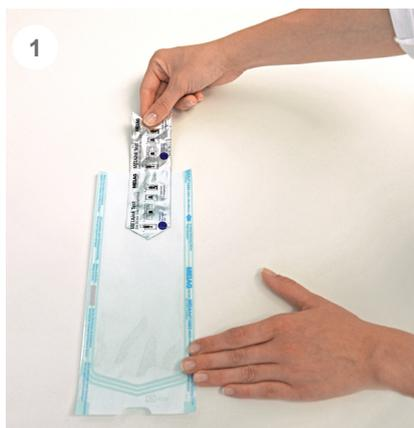
Place the ink test in a transparent sterilization package.
